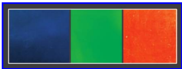
Figure 8. Changes in reflection color of the chiral nematic LC film consisting of 12 wt% of ( R ) E-1 in ZLI-1132 by varying UV irradiation time: 0 s (left), 30 s (middle), and 120 s (right).
